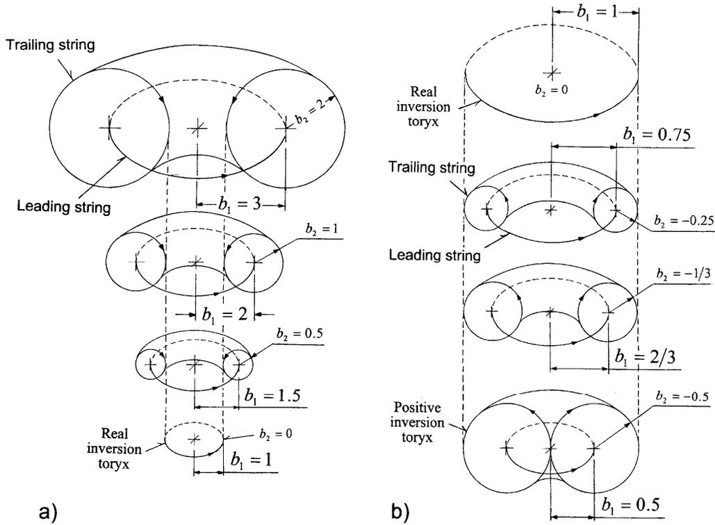
**Figure A28.** Metamorphoses of real toryces: a) negative and b) positive.
