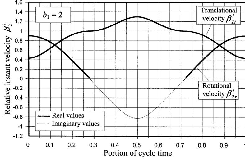
**Figure A14.** Variation of instant velocities  $\beta_{2t}^i$  and  $\beta_{2r}^i$  of the trailing string within one cycle of trailing string.
