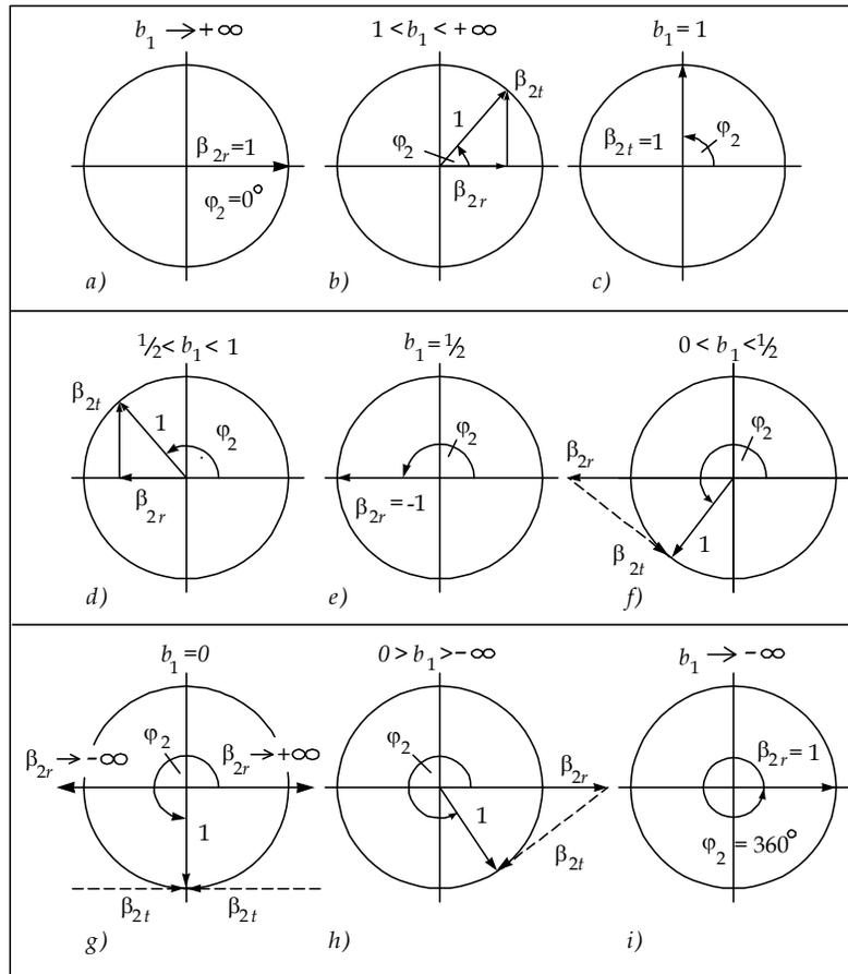
**Figure 13.7.** Velocity hodographs of the toryx trailing string.
